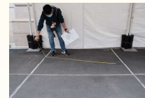
Surveyors conducted visual inspection, measured the length of the cracks on external structures and assessed the structural integrity by suitable instruments.
